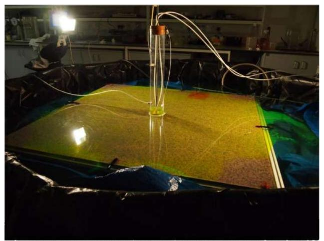
Figure 1. 1.75m<sup>2</sup> granite slab with polycarbonate cover to simulate ~500µm aperture rock fracture with central injection well. Flow paths and flow velocities were measured by monitoring the transport of a conservative (fluorescent green) tracer after each stage of fracture sealing.
